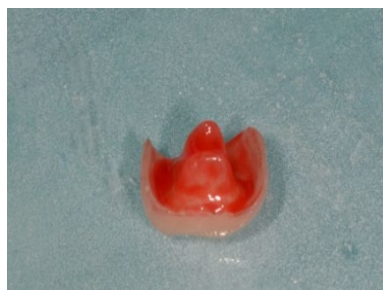
Figure 5. Etching of internal surface with hydrofluoric acid.
